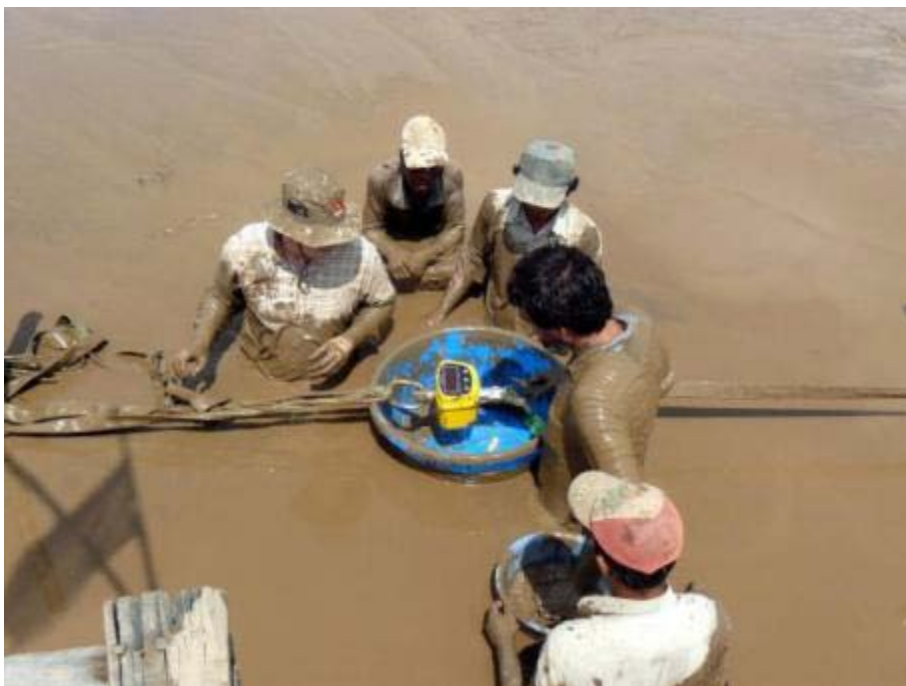
Figure 36: A standard crane weigher is used as a force meter
