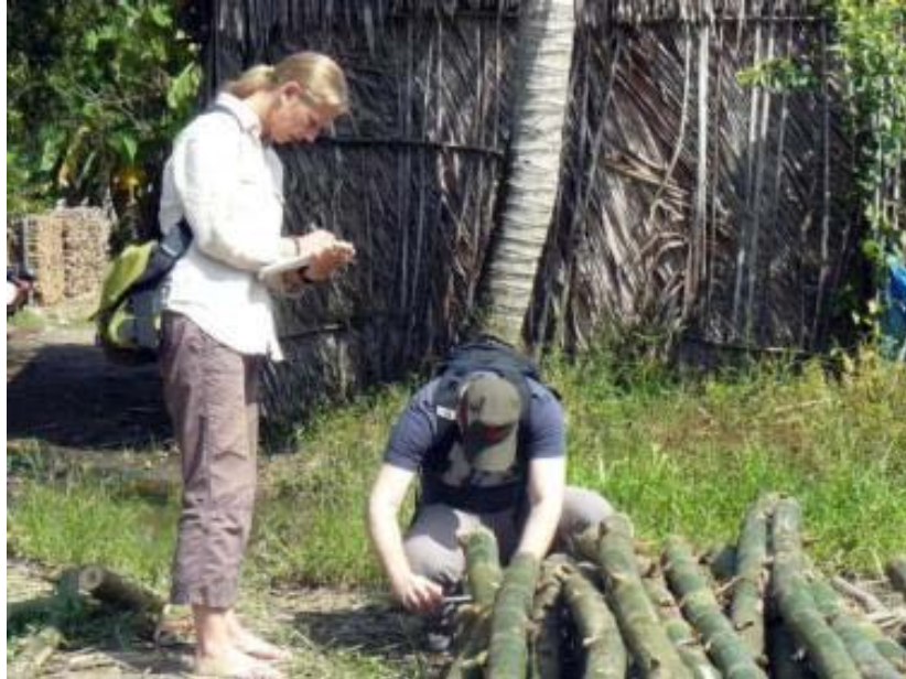
Figure 31: Control of the diameter of the bamboo poles
