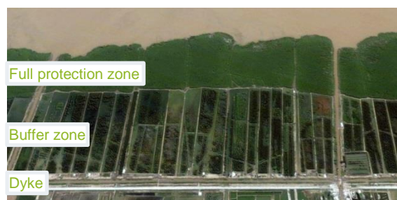
Figure 9: Aerial image of the Mangrove belt in Vinh Hau A. From the bottom to the top: The buffer zone is adjacent to the dike and the full protection zone in front of it by the sea.
