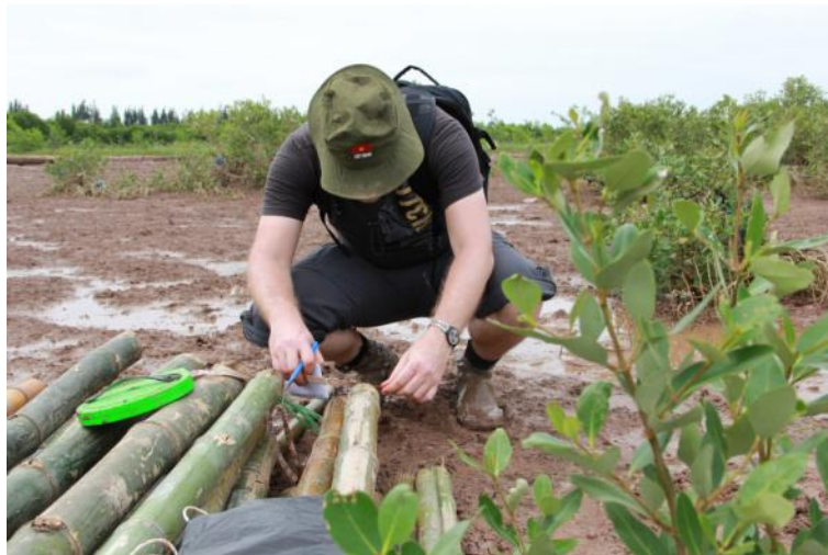
Figure 5: Measurement of the diameter of the installed bamboo
