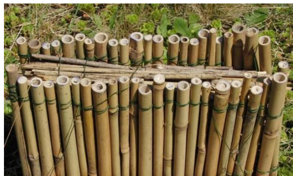
Figure 71: Model of bamboo fence breakwater; filling material between two bamboo rows; top view.
