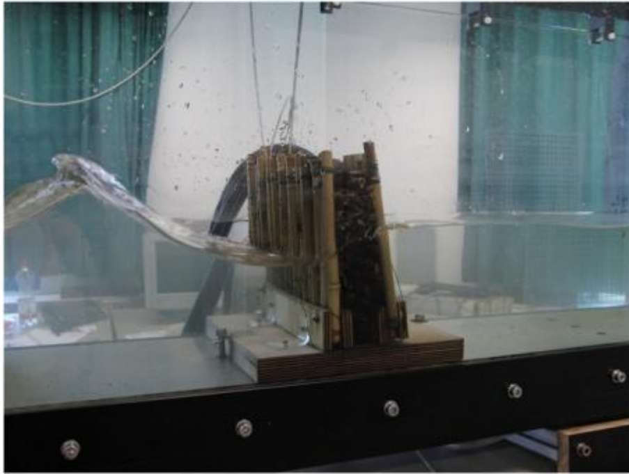
Figure 75: Physical modelling of wave transmission with the bamboo fence.
