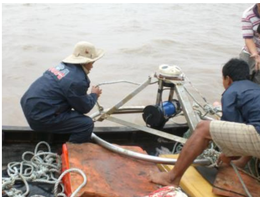
Figure 26: Installation of the AWAC at the coast of Vinh Tan.
