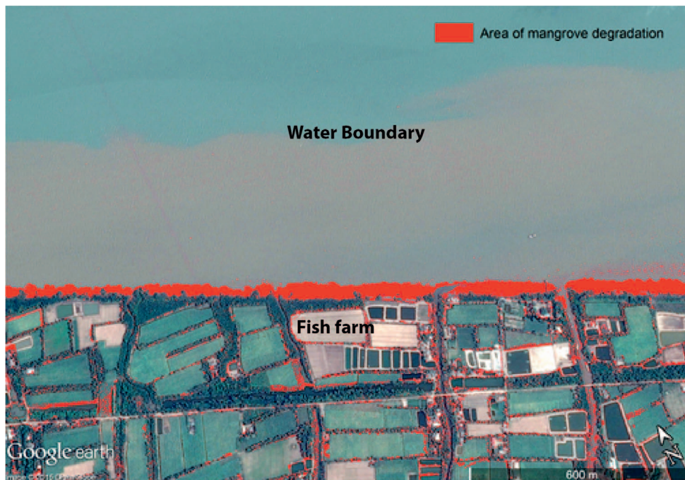
Figure 2. Mangrove degradation along a straight part of Dinh An Estuary in An Thanh province (location 14). The red area illustrates the loss in mangrove area from 2006 to 2014. Fish farms constructed close to the water boundary pushed the mangrove into a narrow fringe zone. This area is suffering from erosion at a rate of about 2.5 \text{ m y}^{-1} .
