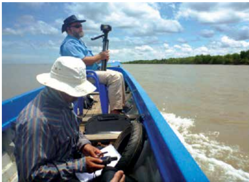
Video operator facing sideways to direction of travel, resting tripod on knees to avoid vibration Observer / Recorder recording GPS waypoint numbers
