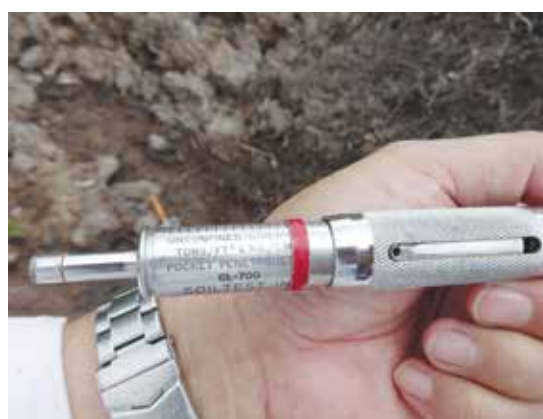
Figure 5: Pocket vane tester with adapter CL 102 (left) and pocket penetrometer (right)
