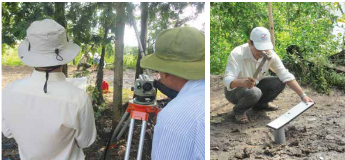
Figure 8: Land survey (left) and soil sampling (right)
