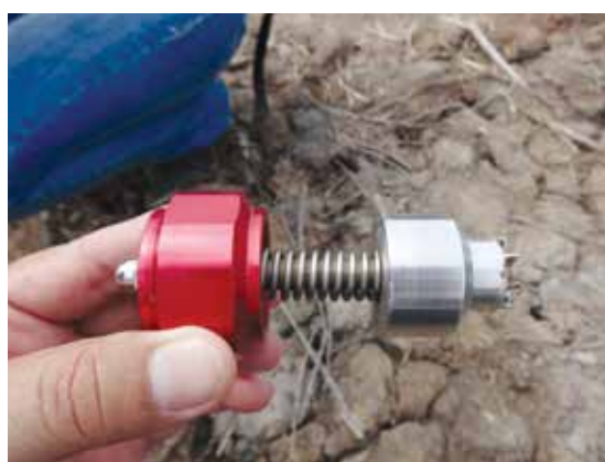
Figure 5: Pocket vane tester with adapter CL 102 (left) and pocket penetrometer (right)
