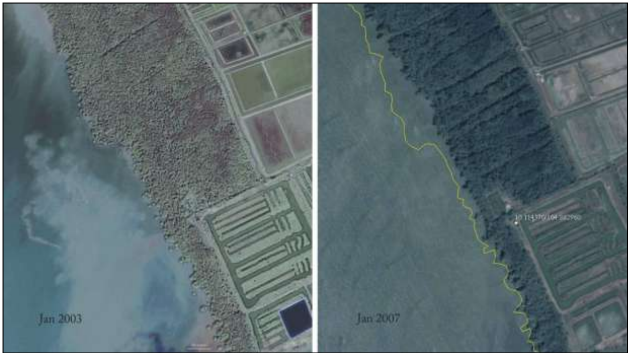
Figure 8: Mangrove retraction between 2003 and 2007 at Hon Queo. Yellow line represents 2003 mangrove front. Note canals cut through forest between dates, plus further loss since 2007 (not shown) (Image: Google Earth).
