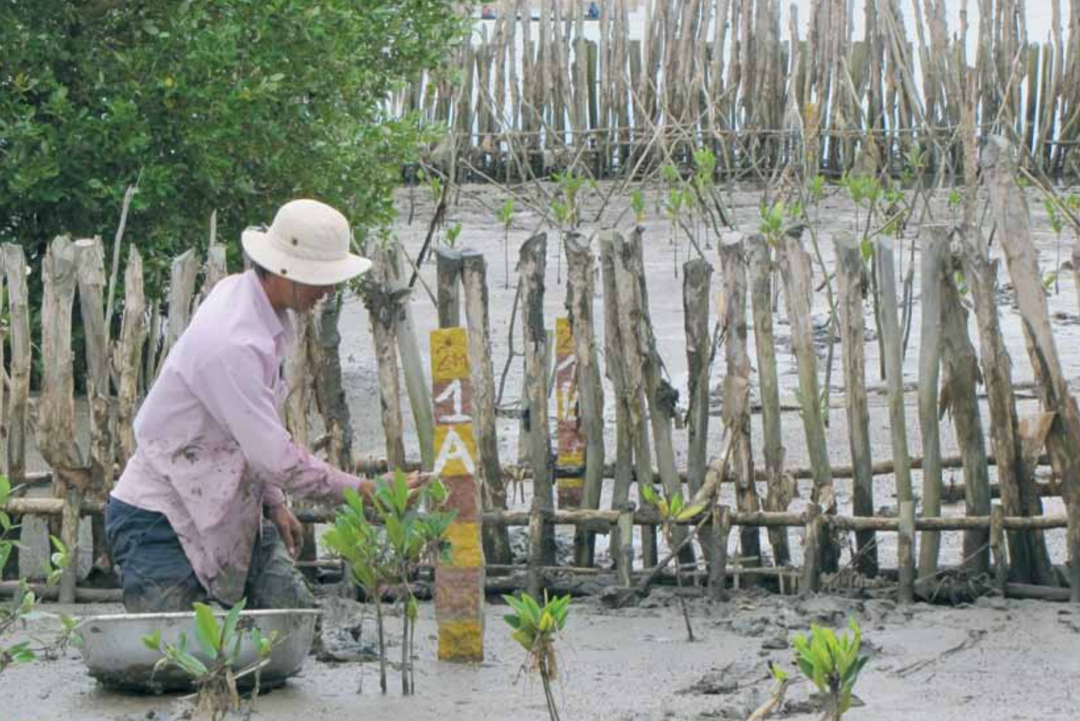
Technician numbering sediment accumulation monitoring pole.
